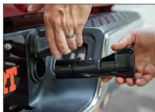
Insert Echo™ between the vehicle and trailer
